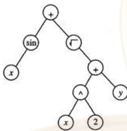
FIGURE 9.1 Program tree representation in genetic programming. Arbitrary programs are represented by their parse trees.
