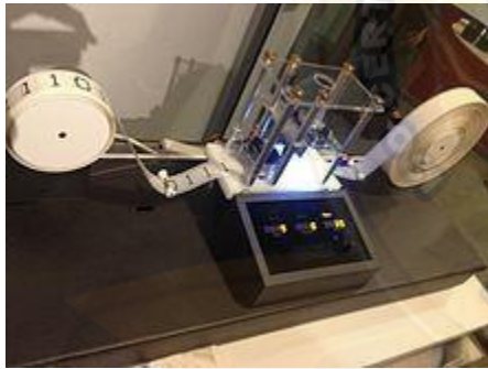
An implementation of a Turing machine
